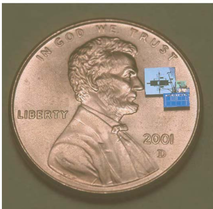
▲ Figure 5-12 Smart dust. The visions for smart dust presume that it will be relatively undetectable by the human eye. Current research efforts have dramatically brought down the size of the dust. (Berkeley)
