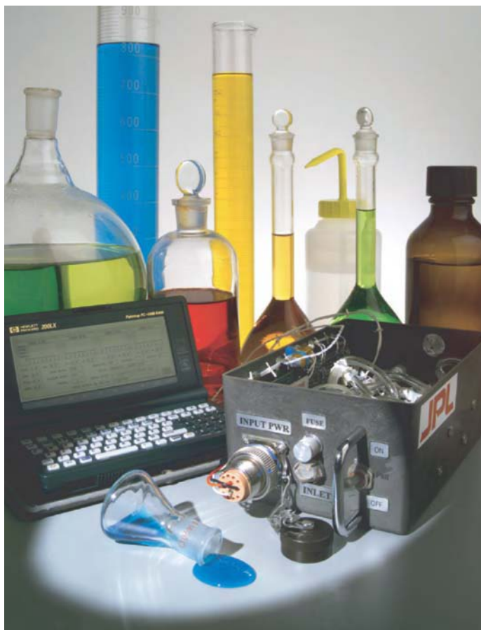
▲ Figure 5-1 This 'electronic nose' contains an array of chemical sensors that swell and shrink, depending on what trace vapors may be present in the air. Measuring this variation allows certain elements in the air to be identified. (NASA)
